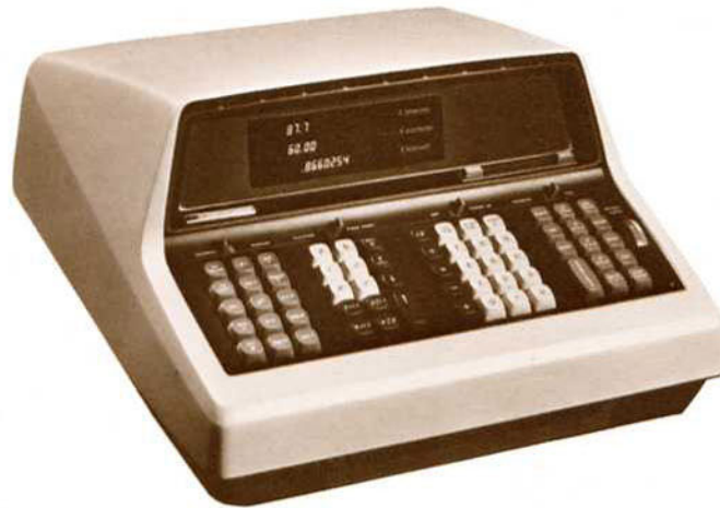
Programmable Desktop Calculator. Introduced in 1968, it is more powerful than the much larger ENIAC and is built with discrete transistors.
