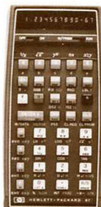
Hand-Held Programmable Calculator. Integrated circuit technology made possible a hand-held calculator more powerful than the desktop calculator pictured above.
