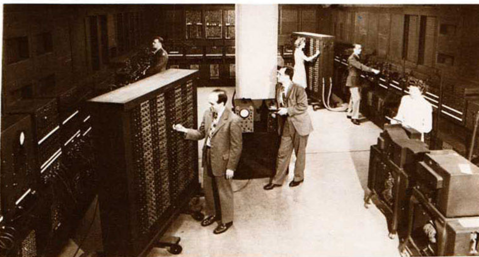
ENIAC Calculating Machine. Built in 1946, it was the first general-purpose electronic computing machine. It used over 18,000 vacuum tubes and required a power supply half the size of the computer itself. (Photo Courtesy UPI)
