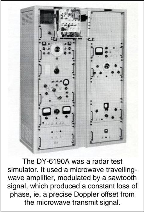
The DY-6190A was a radar test simulator. It used a microwave travelling-wave amplifier, modulated by a sawtooth signal, which produced a constant loss of phase, ie, a precise Doppler offset from the microwave transmit signal.
