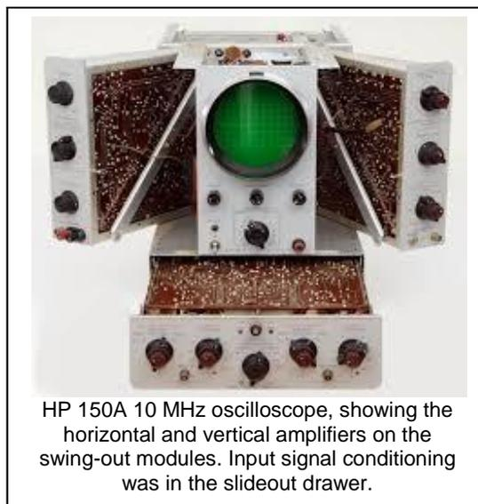
HP 150A 10 MHz oscilloscope, showing the horizontal and vertical amplifiers on the swing-out modules. Input signal conditioning was in the slideout drawer.
