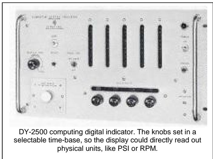
DY-2500 computing digital indicator. The knobs set in a selectable time-base, so the display could directly read out physical units, like PSI or RPM.
