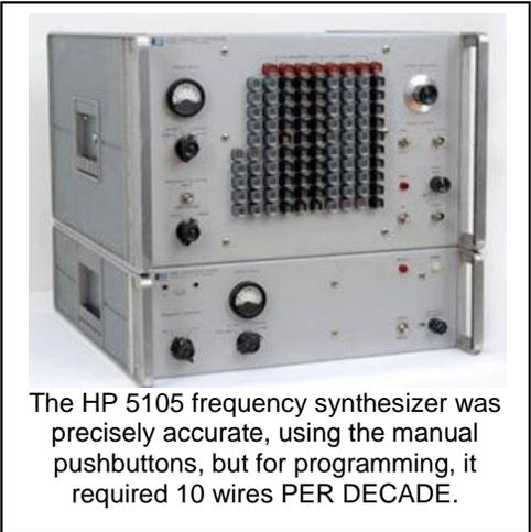
The HP 5105 frequency synthesizer was precisely accurate, using the manual pushbuttons, but for programming, it required 10 wires PER DECADE.
