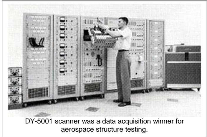
DY-5001 scanner was a data acquisition winner for aerospace structure testing.
