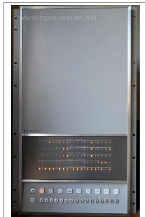
The HP 2116A Computer featured a 16-slot card cage on the lower third, which provided the PC boards which interfaced with measurement instruments.
