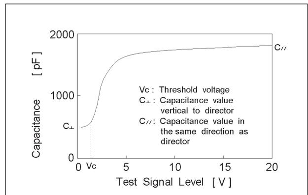
Figure 2. Voltage-capacitance Characteristics Measurement Results
