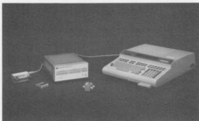
Figure 37. HP 11713A Attenuator/Switch Driver supplies drive power for up to 10 HP 33311B/C Switches under HP-IB program control.
