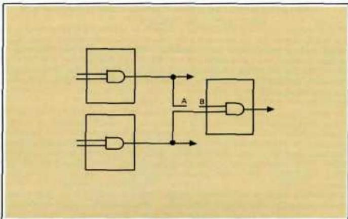
*Figure 9. The Effect of an Open in the Circuit External to an IC. All inputs attached to the node at Point A will be driven properly. All inputs to the right of the open (Point B) will be left to float to a "bad level" and will therefore look like a static high state.*
