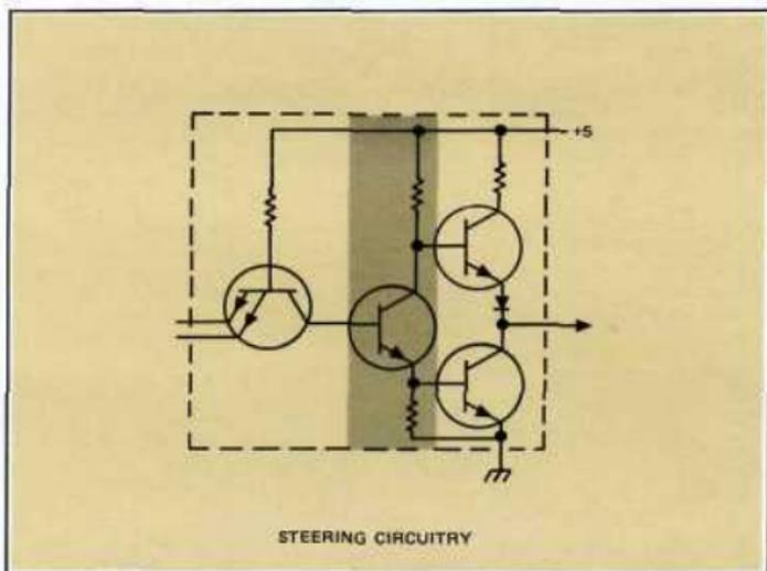
Figure 8. The Effect of a Failure of the Internal Circuitry of the IC Upon Circuit Operation. A failure of the steering circuitry of an IC will either cause the output to be in a static high state or a static low state.
