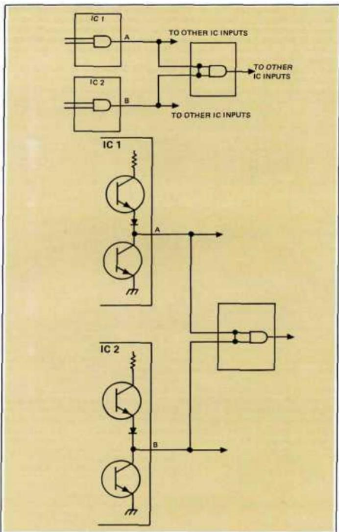
Figure 7. The error effect of a short between two pins occurs when the outputs driving those pins attempt to pull the short to opposite states. In this case, the output attempting to pull the node high will be supplying current while the output attempting to pull the node low is a saturated transistor to ground and will be sinking the current. The saturated transistor to ground will thus pull the node to a low state.
