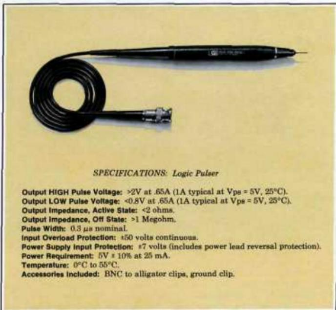
Figure A3. 10526T Logic Pulser. The Logic Pulser provides a solution to the in-circuit stimulus problem of TTL and DTL circuits. Nodes are automatically pulsed from their current digital state to the opposite state for 300 ns with the press of a finger.
