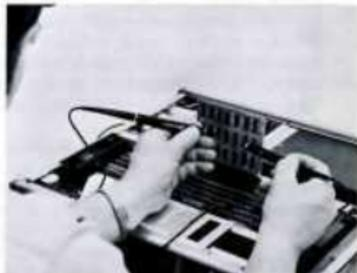
**STEP 4.** Test for a short between two nodes using the Logic Probe and Pulser or an ohmmeter.
