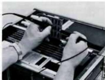
**STEP 3.** Test for a short to Vcc or GND using the Logic Pulser and Probe. By simultaneously probing and pulsing the bad node a short to Vcc or GND can be detected since the Pulser is unable to inject a pulse into such a short.
