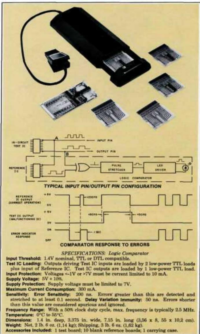
Figure A4. 10529A Logic Comparator. The Logic Comparator uses the test circuits signals to stimulate a reference IC which is mounted on a reference card. The resulting output signals are compared and any differences longer than 200 ns are displayed on the corresponding LED in the Logic Comparator.
