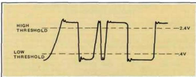
Figure 2. TTL Signal. In the digital world, the relative value of a signal voltage with respect to the threshold voltages determines the operation of the circuit. A signal above the high threshold is in the high state and whether it is 2.8V or 3.0V is unimportant to the operation of the circuit.
