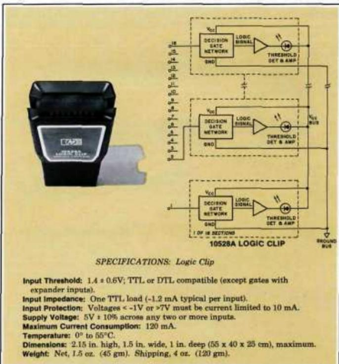
Figure A2. 10528A Logic Clip. With the Logic Clip, up to 16 signals on a given IC can be observed simultaneously. Internal power seeking circuitry allows the clip to be attached in any orientation and makes its operation completely portable.
