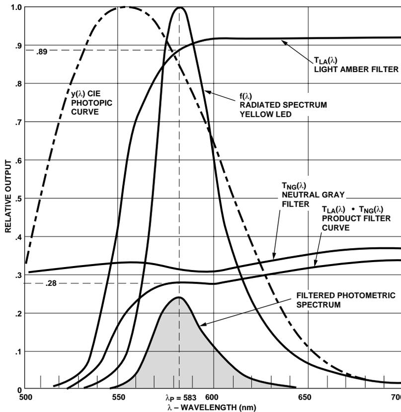
Figure 14. A Neutral Density Gray Filter in Combination with a Light Amber Filter for Use with Yellow Displays.
