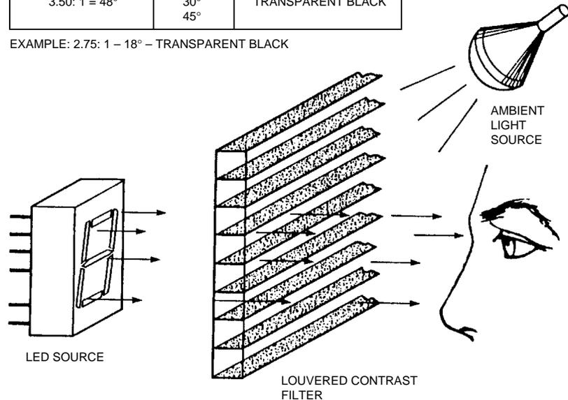
Figure 32. The Operation of a Louvered Filter.
