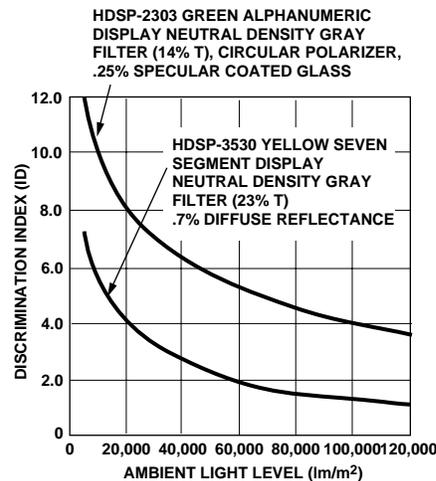
**Figure 47. Effect of Reducing Ambient Lighting.**
