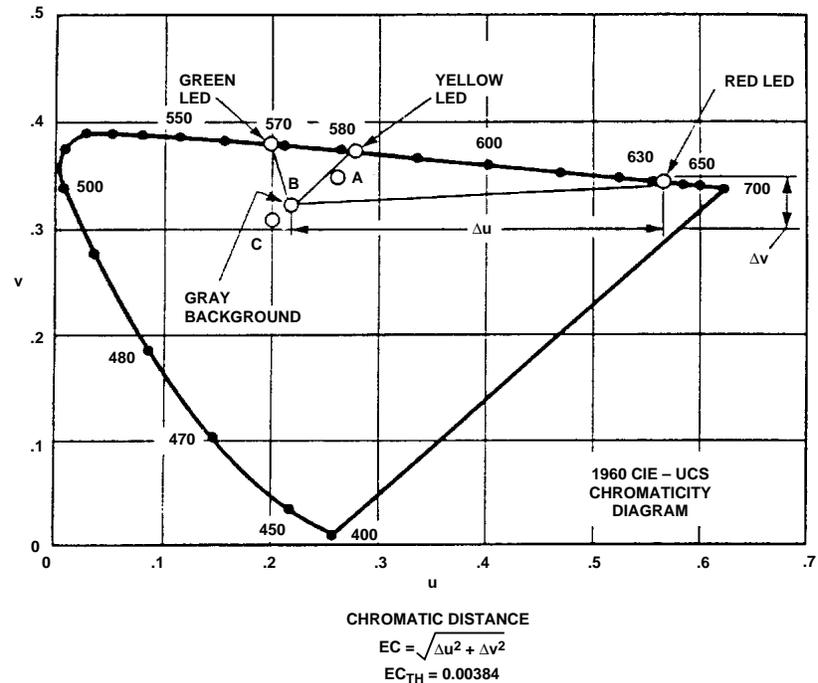
**Figure 21. 1960 CIE-UCS Chromaticity Diagram with the Chromatic Distance Between a Green, Yellow or Red LED and a Gray Background.**
