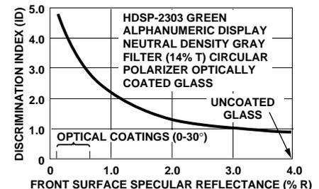
**Figure 45. Effect of Reducing Front Surface Reflectance.**
