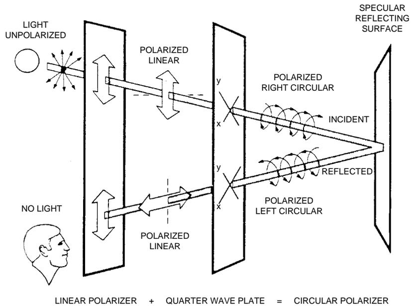
Figure 35. Operation of a Circular Polarizer.
