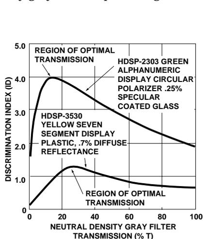
**Figure 46. Optimal Neutral Density Gray Filter Transmission.**
