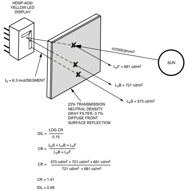
Figure 25. Luminance Index — Diffuse Front Surface Reflectance.
