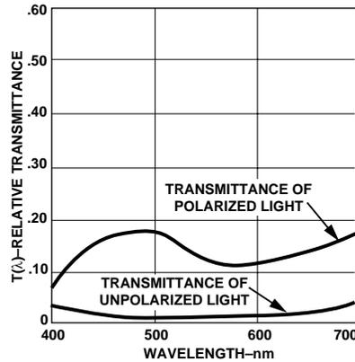
**Figure 38. Spectral Characteristics of a Circular Polarizing Optically Coated Glass Filter.**
