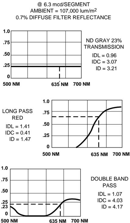
Figure 29. HDSP-3530 High Efficiency Red 0.30 inch Display.
