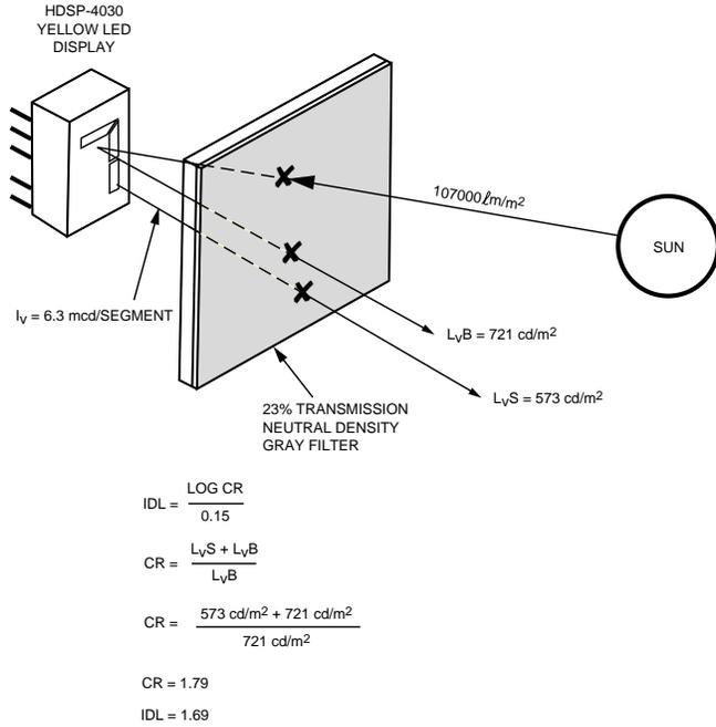
Figure 24. Luminance Index — No Front Surface Reflectance.
