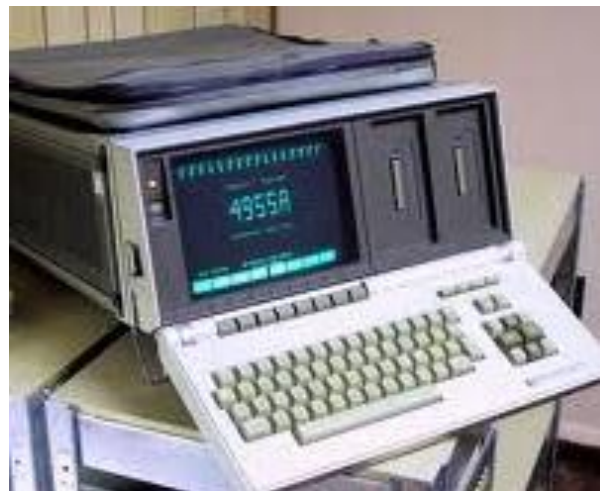
A typical Datacom product, the HP 4955A Protocol Analyzer served research as well as network maintenance, such as computer room performance.
