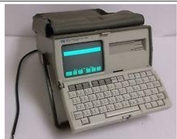
This portable HP 4951A Protocol Analyzer went out in the field for network installation, qualification and maintenance.
