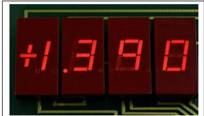
This clever design not only reduced the LED die count to 9 (2-dots), but featured an optical reflection method to stretch the illumination of one die to a full linear segment. .
