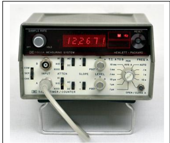
HP 5300A Frequency Counter. It was fully portable, with snap-on-bottom signal processors. It featured a 4 x 7 array of LED die.
