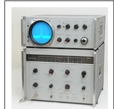
The HP 8551/851 Spectrum Analyzer was our first blockbuster product in 1965. It became the grandfather for half of the Santa Rosa Division.
