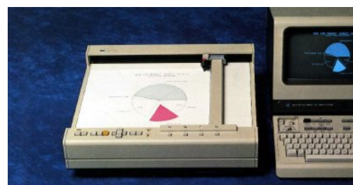
HP 9872A Plotter. This was the period in industrial product design where hundreds of drafting tables were being replaced by pen plotters and computer assisted design software.
