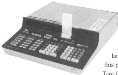
This is the 9820A, one of many in a line of desktop calculators to follow the 9100A.
