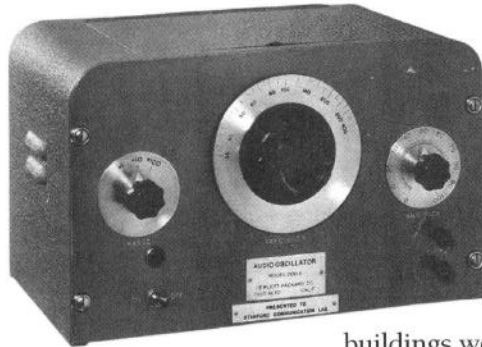
The Model 200A was the world's first low-cost, practical, R-C tuned audio oscillator with its output level controlled by a feedback loop consisting of a simple incandescent light bulb.
