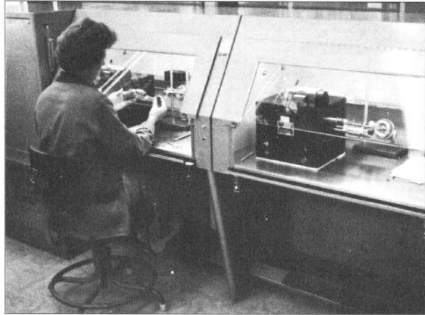
Hazel Benesh winding resistors at the Components Building for the 3440A Digital Voltmeter, one of several products to use this type of component.
