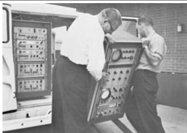
Lyle and John Smylie of the Southwest Sales Division show how spectrum analyzer demonstrator rack can be moved into a customer's plant. From Measure Magazine, December 1964
