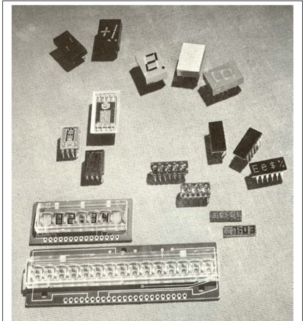
OED visible LED optoelectronic products: Top: 0.03 inch and 0.43 inch character S4 Displays Left center: HDSP-7300 and -7010 Dot matrix OBIC Displays Center: Monolithic calculator displays Center right: HDSP-2000 SAN displays Lower left: PC board displays.
