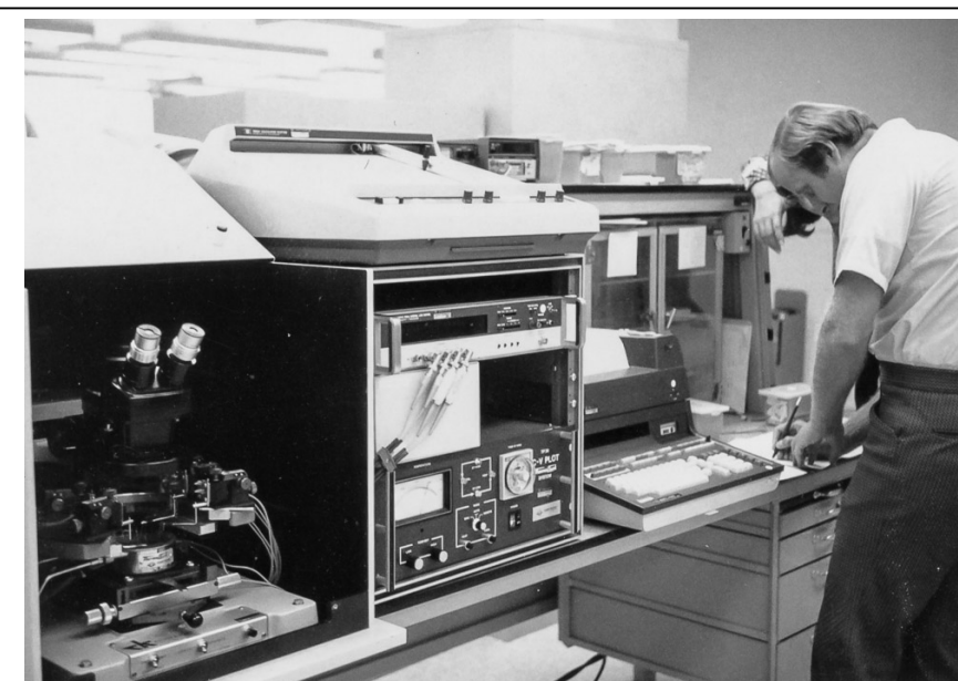
Automated CV Plotter designed and programmed by Chris Clare to automatically measure, plot, and analyze CV curves for characterization of mobile ion drift in oxide layers. Dr. Fred Schwetmann studying his results in ICPL.
