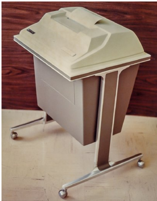
ES Line Printer Built in HP Labs with printout detail 80 character line, 10 lines/second, and full graphics
