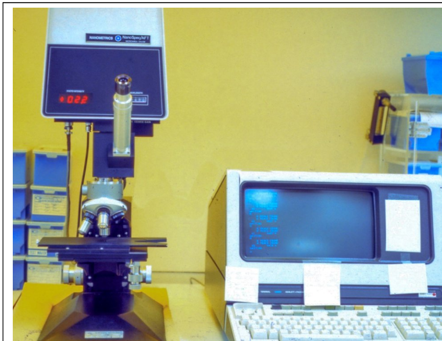
Special Serial Interface was added to a Thin Film Measurement Tool by Nanometrics Readings appears on PCS Terminal to right.
