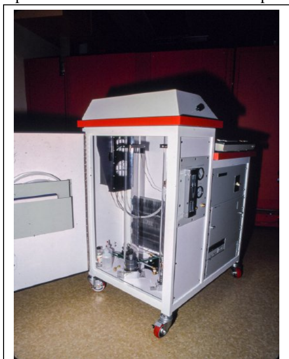
Computerized Mass Flow Controller Calibrator built by ICPL Automation Lab.
