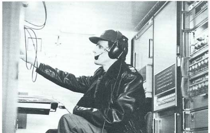
Ground support technician calls up test program at autotester control panel.
