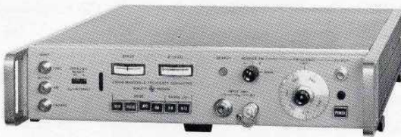
Latest of Dymec's phase-lock instruments, DY-2590B Microwave Frequency Converter is versatile microwave measurements tool.
