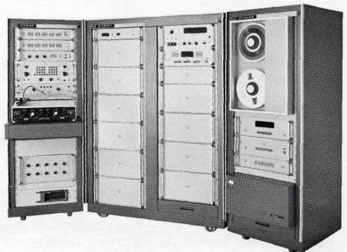
Example of standard 2010 system (1965) expanded to 2000 channels, with on-line plotting capability.
