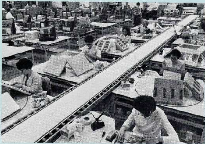
Photo shows main printed circuit loading line. Conveyer belt brings parts to women as well as delivering loaded boards to soldering area.
