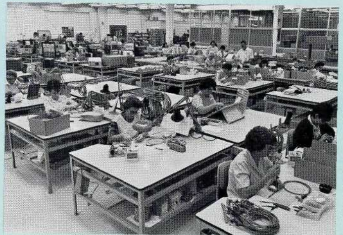
New benches are designed to make cable harness manufacture convenient and efficient. This arrangement is designed to handle current volume smoothly, is easily expanded for future growth.
