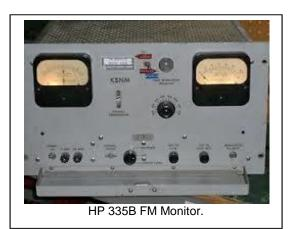
that you could measure the spacing between the video and the oral carriers, and display them on a meter. It's nominally about 4.5 megahertz. The FM circuits of the monitor were fairly straightforward, except that we used more modern parts than we had on the earlier ones. We also had a little bit more packaging on the thing.
