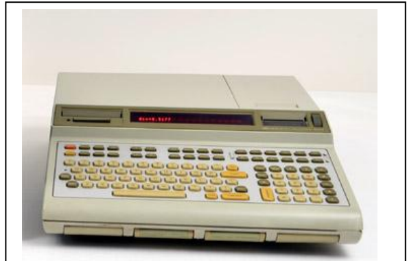
The HP 9825A Desktop Calculator was the first major HP project to use the SAN displays. Since it featured powerful programming functions, the alpha characters were required.
