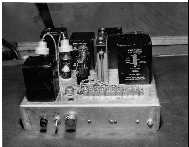
Dual power supply for pulse amplifier and photomultiplier
