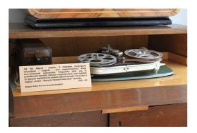
Two pictures show the tape recorder adapter and its electronic control box. The adapter used a conventional record player's electric motor, saving the driving mechanism's cost.
